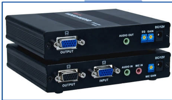
VGA/Audio Extender Kit - Includes transmitter, receiver and power adaptors. (SKU: VAC5-E for 180Meters and VAC5-EP for 300Meters)
